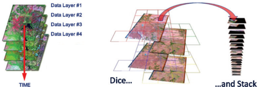
Figure 1.3 Schematic illustrating how satellite image data cubes work
