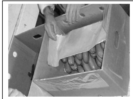
Figure VII.2.1. Paper lining material used to pack bananas in order to prevent abrasion damage during handling and transportation
