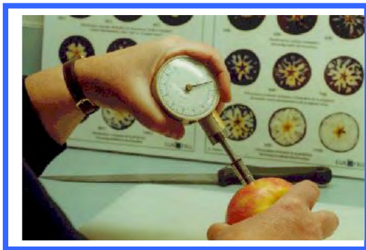
Fruit firmness tester for apples
