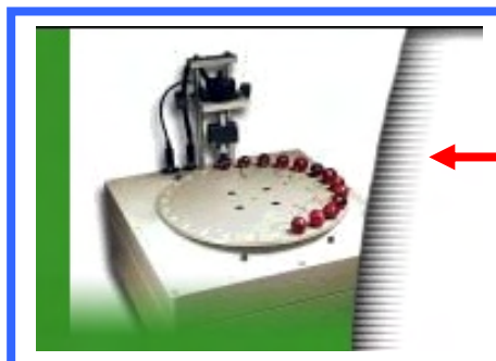
Fruit firmness tester for apples
