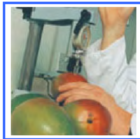
Firmness tester for mangoes
